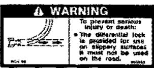
Locate on Panel Above Differential Lock Pedal (Part No. 901938)
