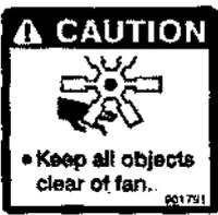
Locate on Left and Right Side of Radiator (Part No. 901791)
