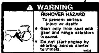
Locate On Side Panel Above Clutch Pedal (Part No. 901935)
