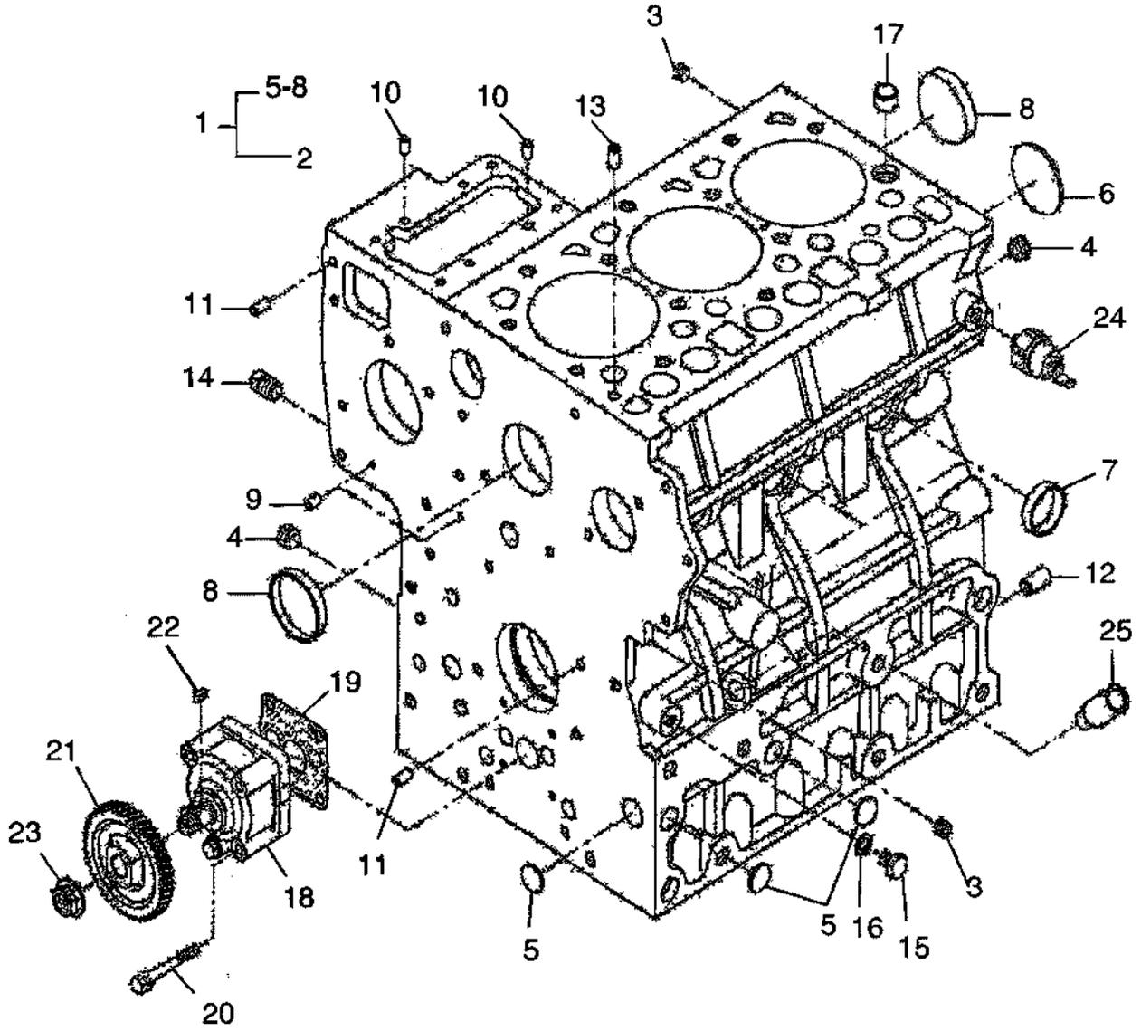
**CYLINDER BLOCK (270 DTC)**
